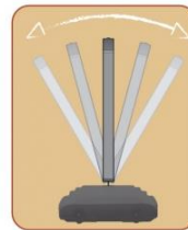
Heavy-duty coil springs resist strong winds and return the sign to an upright position
